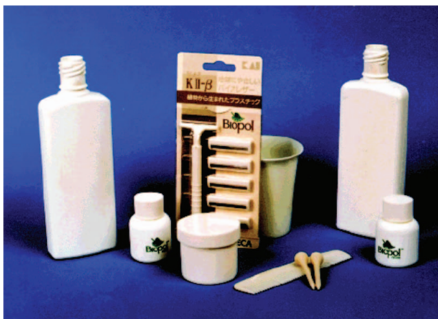
Figure 3. Moulded PHB objects for various applications. In soil burial or composting experiments, such objects biodegrade in about three months [2].
